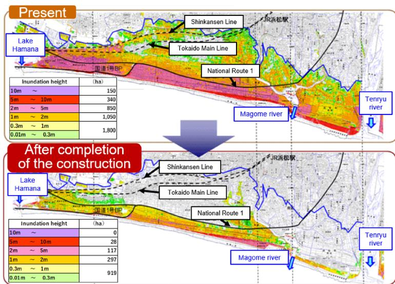
Fig.1 Effect of embankments against the Nankai Trough Earthquake tsunami in Hamamatsu
